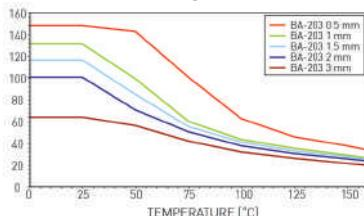
$\sigma_{BO}$  diagrams represent  $\sigma_{BO}$  values for different gasket material thicknesses. These values indicate the maximum in-service compressive pressures which can be applied on the gasket area involved without destroying or damaging the gasket material.
